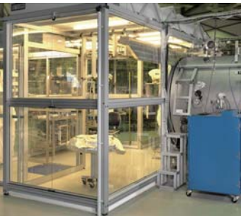
Photos: Site (top); Experimental hall at the Metrology Light Source (MLS); Local clean room and reflectometer for the characterisation of EUV optics – © PTB
